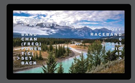
For BetaFlight flight controller firmware above BetaFlight 4.1.0, you need upload a VTX Table to the flight controller before using the remote control to modify the video transmitter parameters normally.
