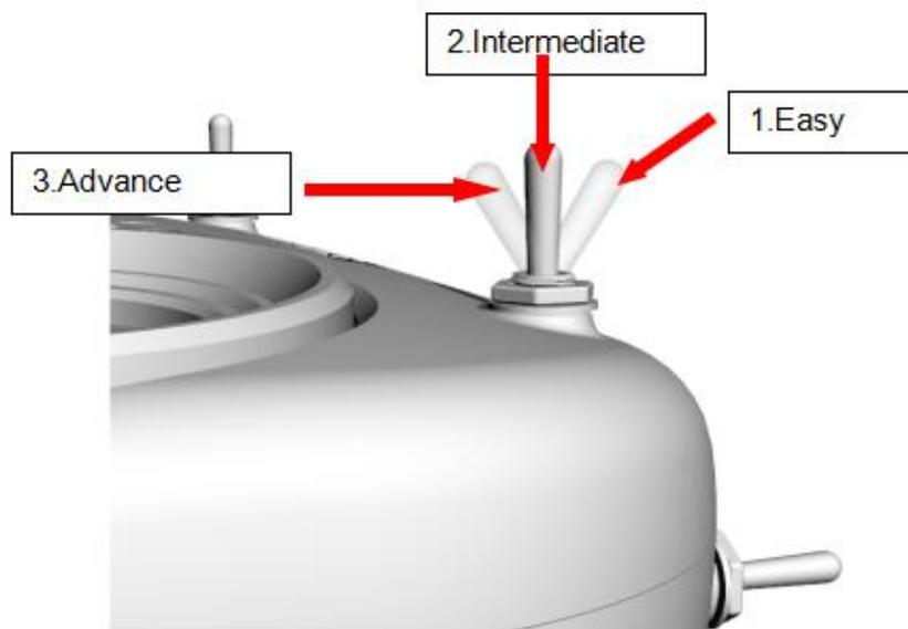
The EZ Pilot Pro is factory set to rate mode. This is an advance mode that sets the angular rate that controls the plane. The AUX 2 switch is set as a 3-level switch that changes this mode. When AUX 2 is in 1st gear, EZ Pilot Pro will be in easy mode to control and set the attitude of the aircraft. When the switch is in the middle 2nd gear, the EZ Pilot Pro will be in the middle mode and the last 3rd gear is the advanced mode.
