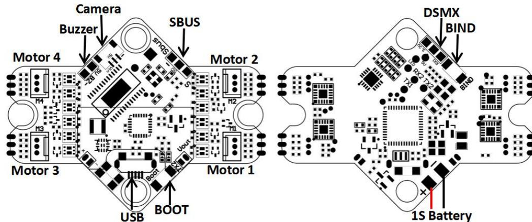
This flight controller has a MCU with a gyro.
